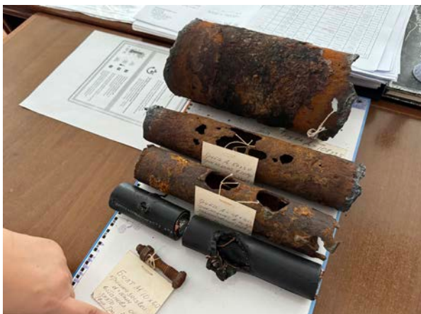
Figure 7: Examples of corrosion in water and heating supply pipes
