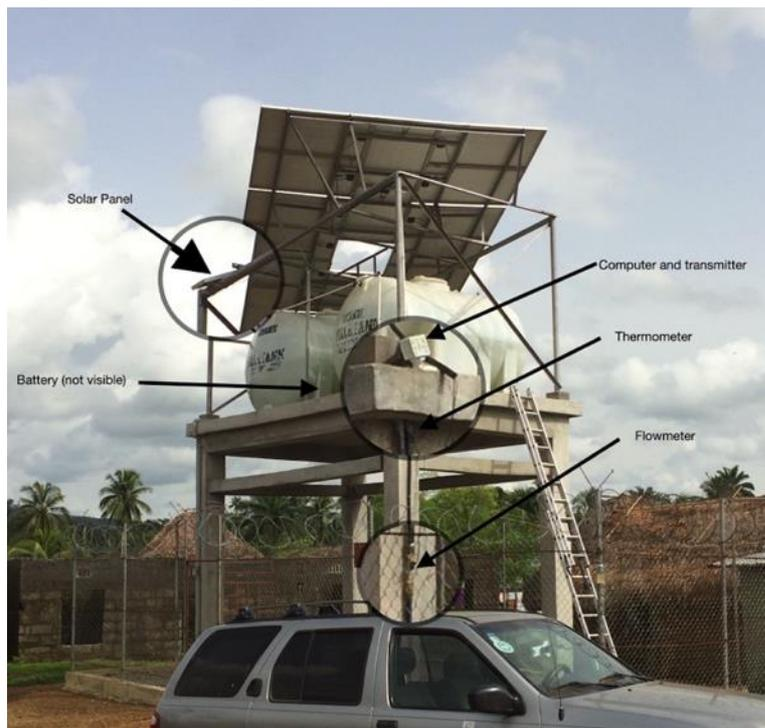
*The solar powered satellite and Arduino device, WASH MONITOR 1, is installed and in operation in Gandorhun.*
