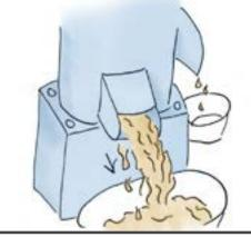
The Finic Machine does the job and produces the palm oil. It drips a little in the other bowl. To avoid waste the users will make sure to pour it over the bowl with the oil.
