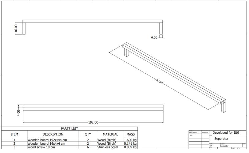
Figure 43. Separator schematics
