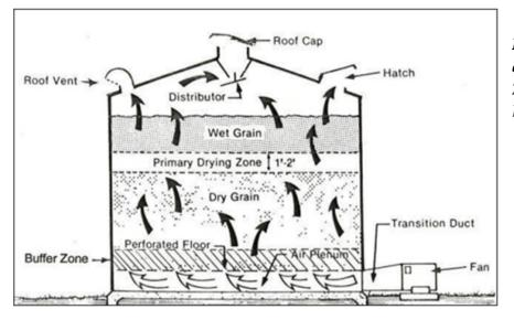
*Figure 13. Batch grain dryer schematic* Encon 2.3. 2012). Improving Energy Efficiency in Grain Drying.
