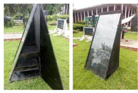
Figure 17 and 18. Solar Grain dryer university of Dhaka Biswas, P. K., Milon Uddin, Huque, S., & Nasif Shams. (2017). Design, Construction and Performance Study of a Low Cost Solar Dryer for Food Preservation in Bangladesh. Institute of Energy, University of Dhaka.
