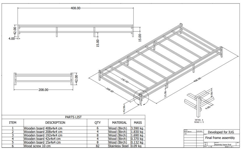
Figure 42. Drying bed Schematics
