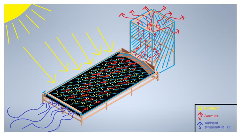
Figure 41. Conveccion of currents in dryer
