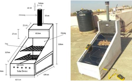
*Figure 19 and 20. Solar Grain dryer University of Dhaka Khan, M., Sengar, N., & Mahavar, S. (n.d.). Fabrication and testing of a low cost passive solar dryer.*
