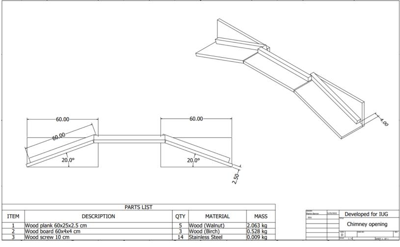
Figure 42. Chimney opening schematics
