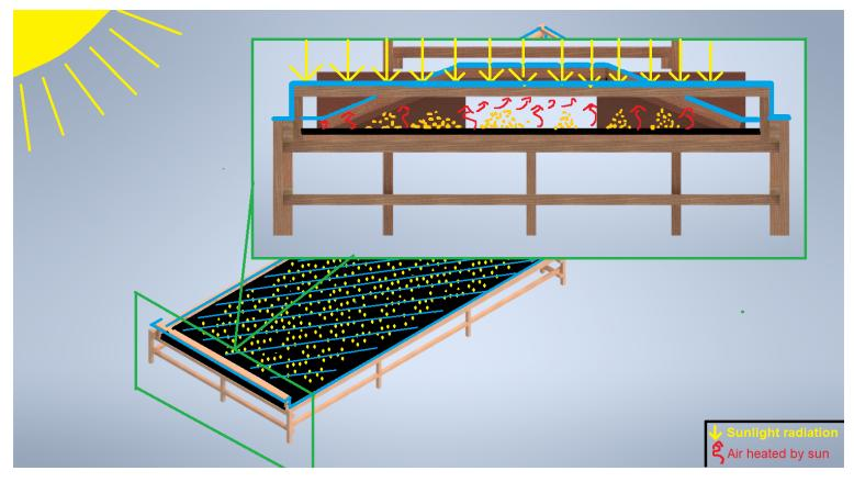
Figure 40. Heated air pocket
