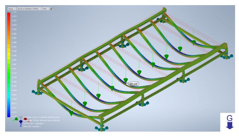
Figure 36. Stress simulation results
